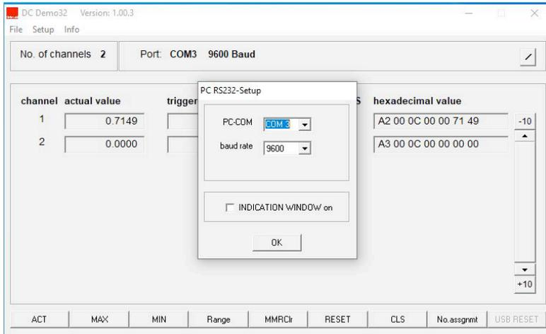
In the “Setup” menu, activate the “DC-Hi-Net Interface Setup” subprogram.
