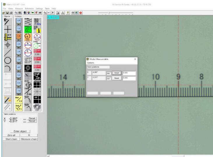
If an incorrect value is displayed for the measurement section traversed, the interpolation of the interface must be set up again. The procedure is as follows.
