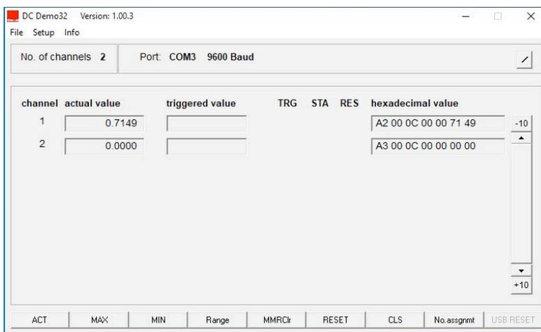
For “Setup”, go to the RS 232 Setup item and select the correct COM connection. The connection will be created and the data transmitted.
