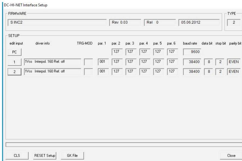
In the next step, go to “Edit/Input 1” and enter the value 005 into Par 1. You now have the correct interpolation for the built-in measuring systems. Then accept / save values.
