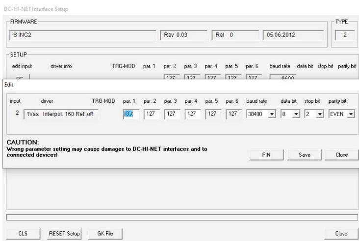
The measuring system display in the metric will now be displayed as plus in the rightward direction of movement and as minus in the leftward direction of movement. Should this be in the opposite direction, then you need to change the interpolation by entering the value 037 into Par. 1 and Par.2. Then accept / save values.
