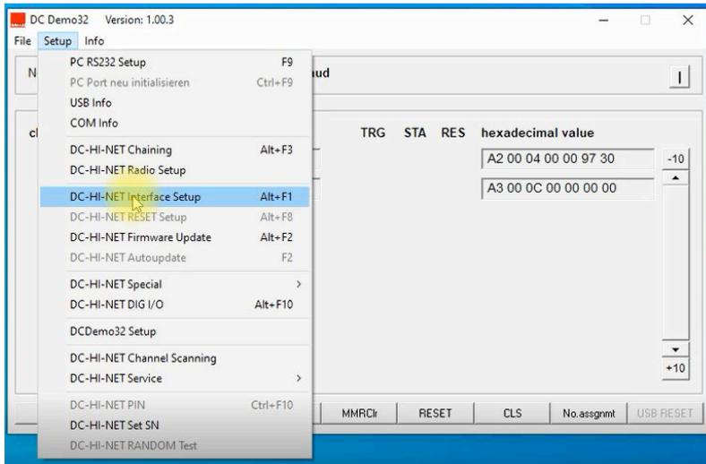
This opens the window containing the configuration data and values. You now need to set the relevant channels so that the values match the measuring systems.
