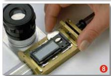
8 Insert new battery («+»-pole looking upwards)
