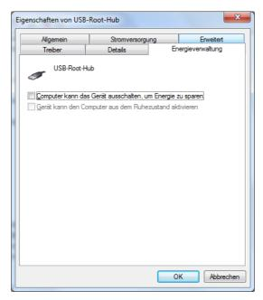
Make sure that the box for 'Allow the computer to turn off this device to save power' is not checkmarked, in other words, that this function is disabled.
