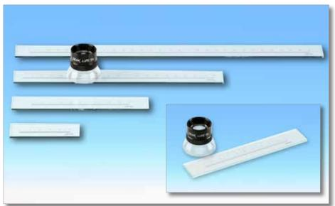
Measurement of greater distances with measuring magnifiers is possible only to a limited extent due to the length of the scales. PEAK glass measuring rods are the optimum supplement for quick and simple determination of lengths and distances. The five lengths of 50 mm, 100 mm, 200 mm, 300 mm and 400 mm are supplied with a 15x reading magnifier (standard 1962 magnifier) in a transport box. When measuring
