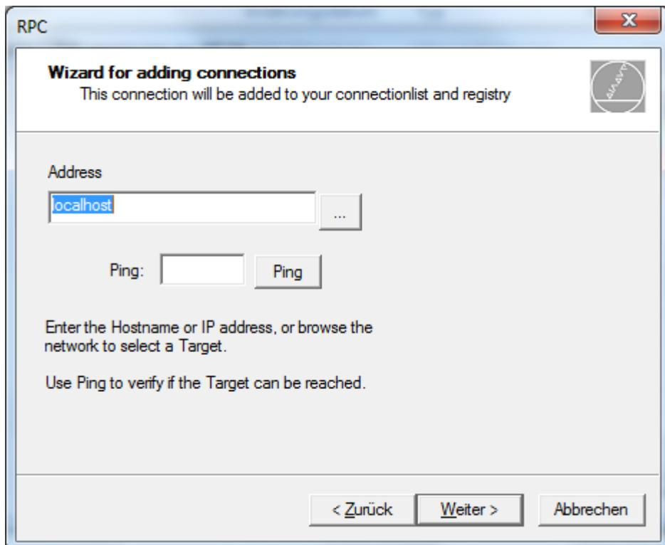
Enter the network connection. If necessary do a ping test to test the availability of the controller. Then click "Next".
