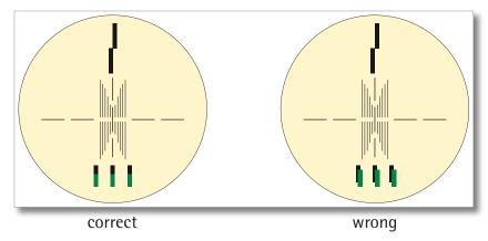
The measurement error increases with the distance between the measuring mark on the reticle plate and the line to be measured on the test material and with the angular deviation of the viewing axis from the vertical.
